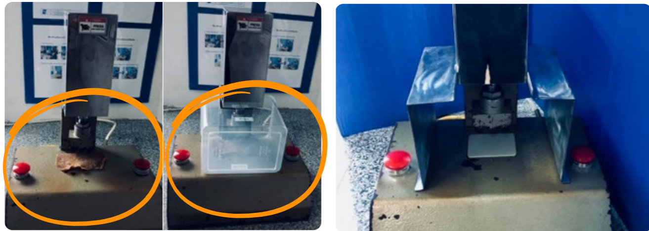
Before: Without safeguard & with temporary safeguard
